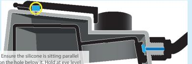
on the hole below it. Hold at eve level to check the position is correct
