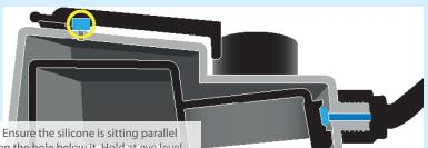
Ensure the silicone is sitting parallel on the hole below it. Hold at eye level to check the position is correct
